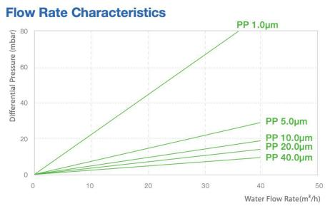
Test Criteria: Single filter (40inch length)cartridge, water at 20°C.
